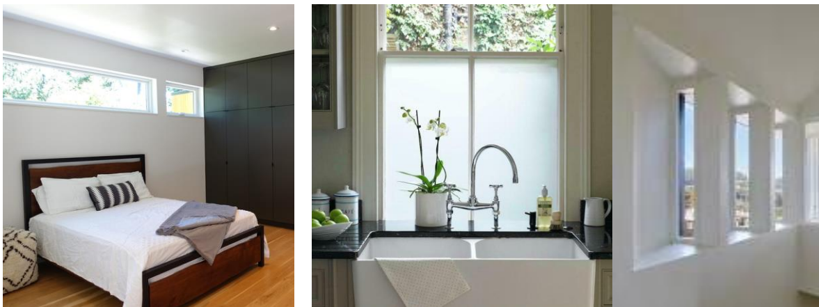
Examples of windows above 5-foot eye level (left), obscured glass below 5 feet (middle), and angled windows (right).
