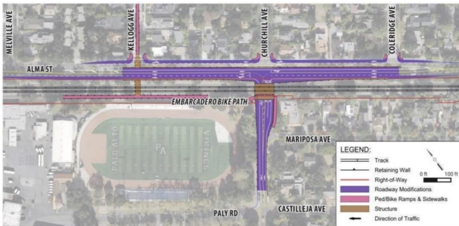
Figure 7. Churchill Avenue Partial Underpass
