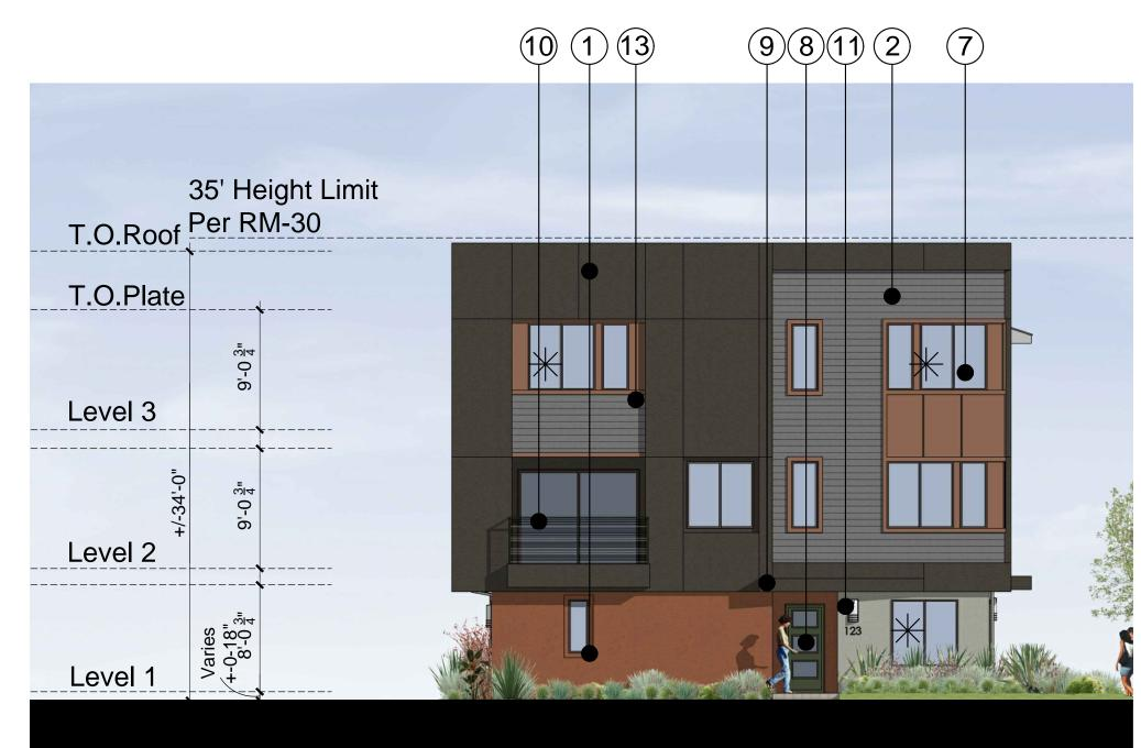
SIDE ELEVATION A (PLAN 3)
