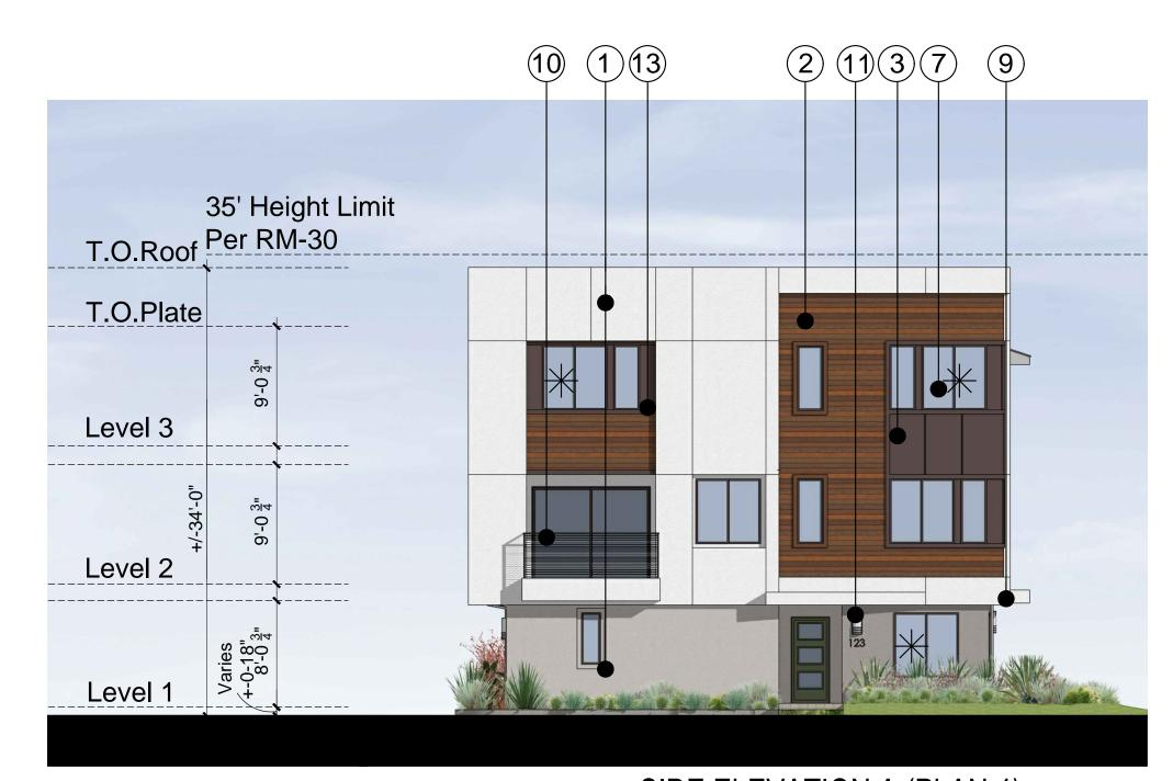
SIDE ELEVATION A (PLAN 4)
