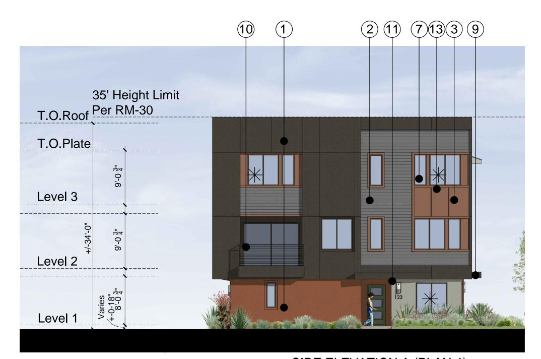
SIDE ELEVATION A (PLAN 4)
