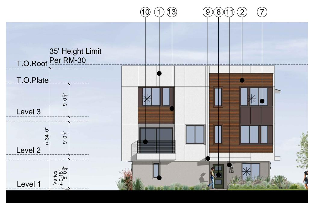
SIDE ELEVATION A (PLAN 3)
