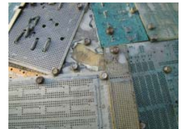
Detail of circuit boards. Note exposed fiberglass, coating failure and mild corrosion at fasteners.
