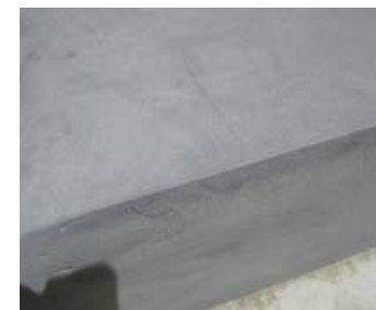
Detail of crack in side of fiberglass base.
