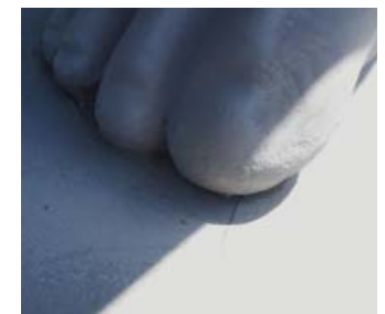
Detail of crack in fiberglass base near toes.
