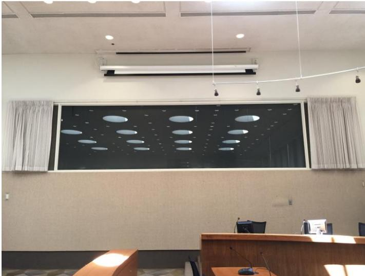
Figure 6 – Example no. 2 of display with overhead glare due to daylight.
