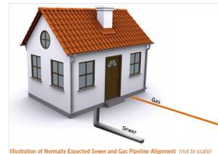
Illustration of Normally Expected Sewer and Gas Pipeline Alignment (not to scale)
