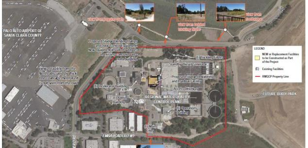
The above aerial indicates the proposed location of the sludge dewatering and loadout facility just southeast of the incinerator building. The new building and truck access route will be placed on land that is currently open with no permanent structures. Other on-site functions
