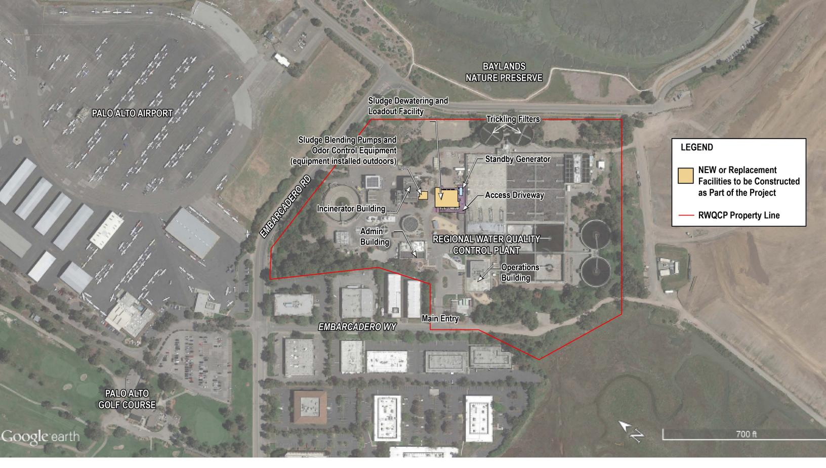
AERIAL PHOTO – EXISTING CONDITIONS AND LOCATION OF NEW SLUDGE DEWATERING & LOADOUT FACILITY PALO ALTO REGIONAL WATER QUALITY CONTROL PLANT
