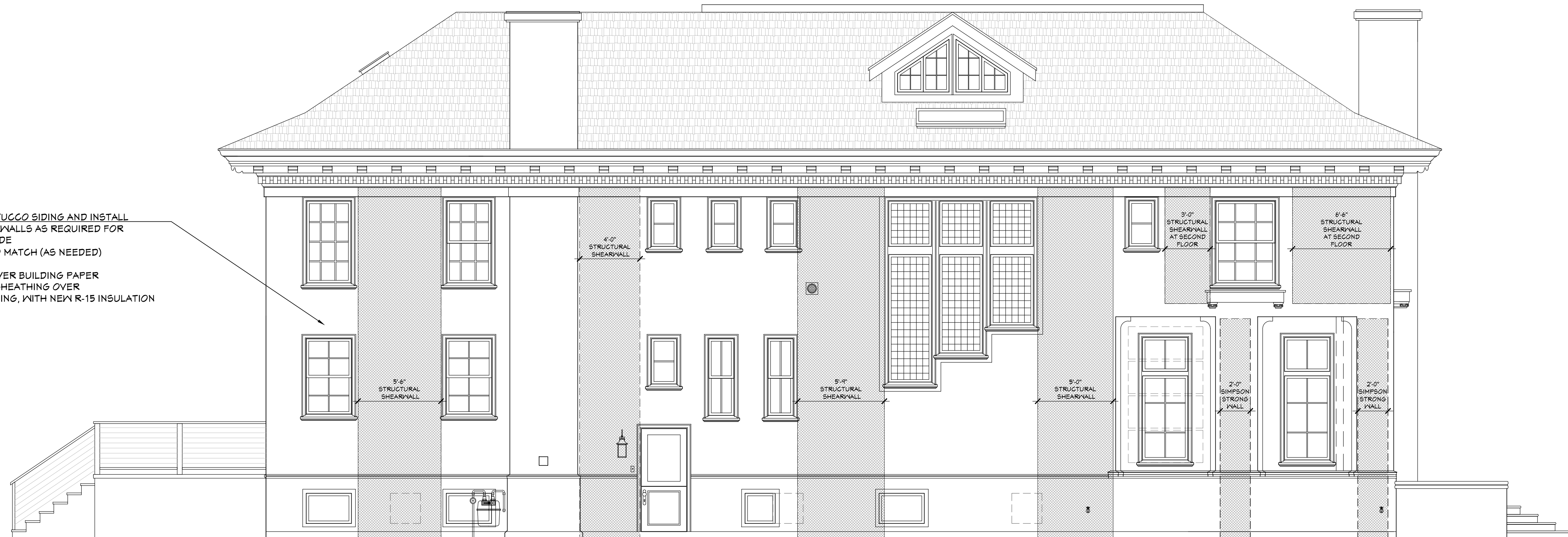
SHEARWALL LOCATIONS DRIVEA SIDE (NORTHWEST) ELEVATION scale: 1/4"-1'-0"
