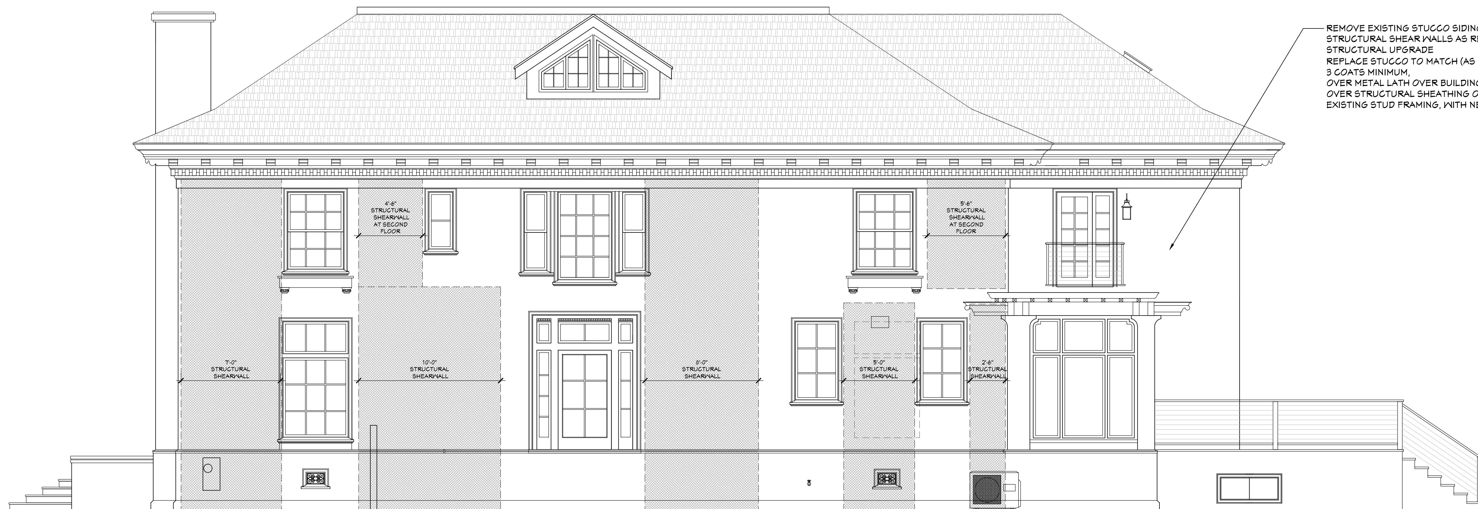
SHEARWALL LOCATIONS INTERIOR SIDE (SOUTH EAST) ELEVATION scale: 1/4"-1'-0"
