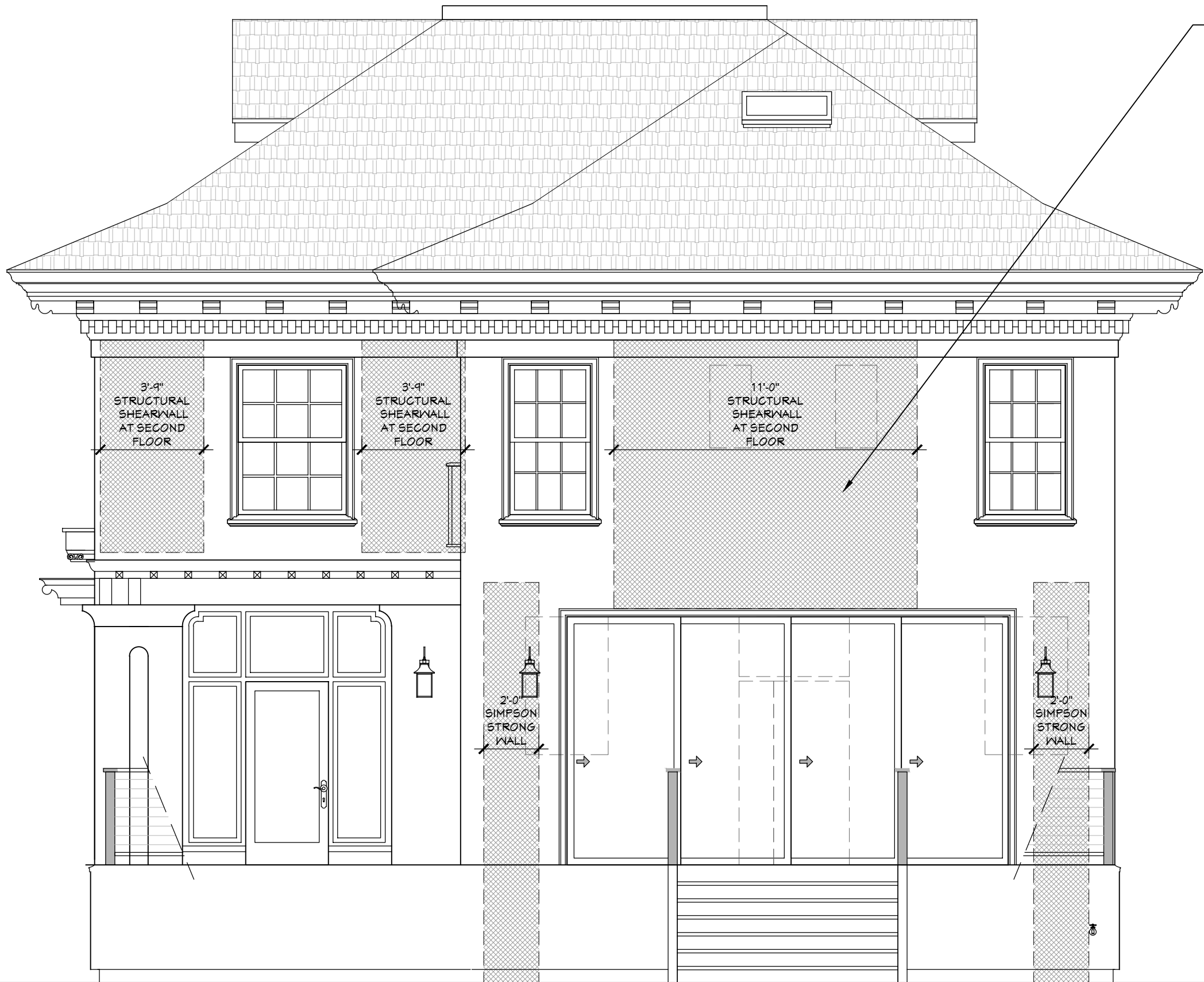
SHEAR WALL LOCATIONS REAR ELEVATION scale: 1/4"-1'-0"
