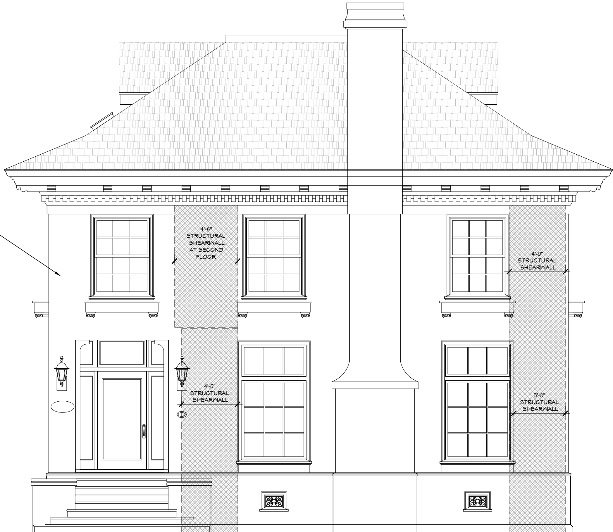
SHEAR WALL LOCATIONS FRONT ELEVATION scale: 1/4"-1'-0"
