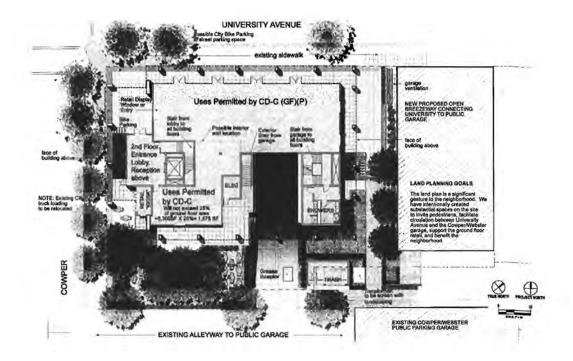
a) The "armature" leg has been pulled back to open the retail arcade on both ends. There is 6' clear between the back of the column and face of retail glass. Please see Sheet A2.1.
