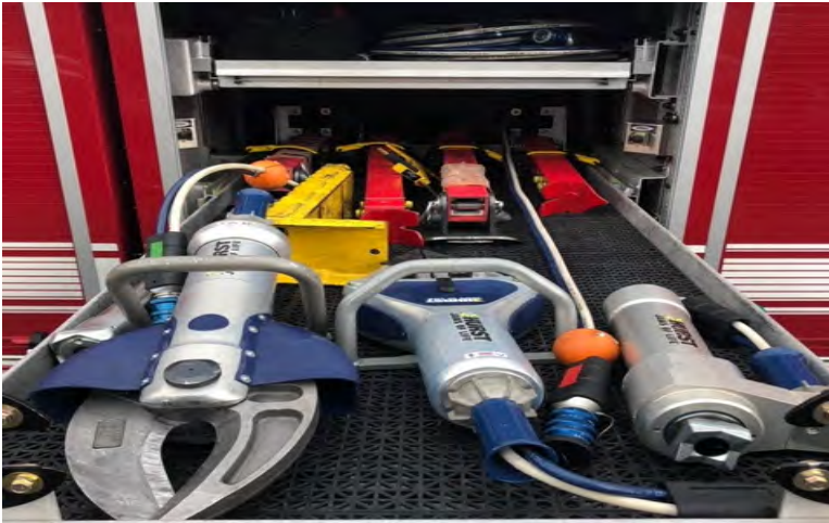
Extrication tools stored on the fire engine
