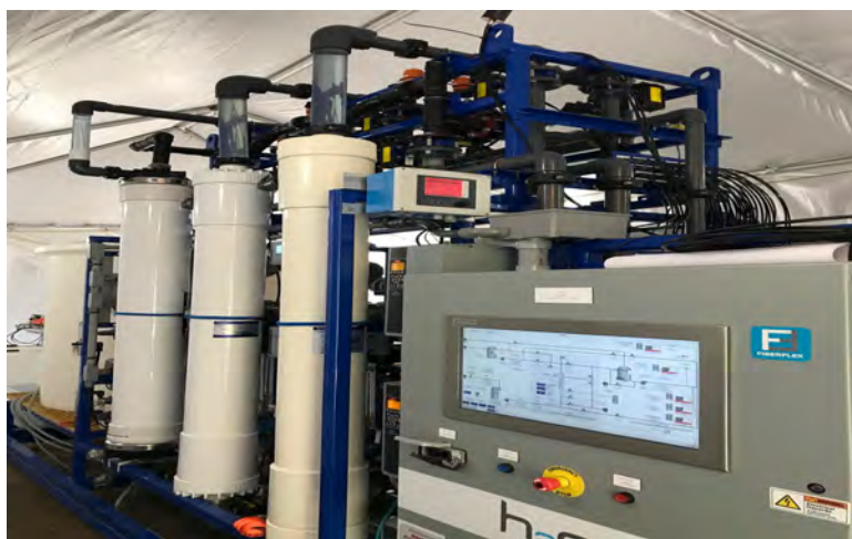
Filtration system testing unit
