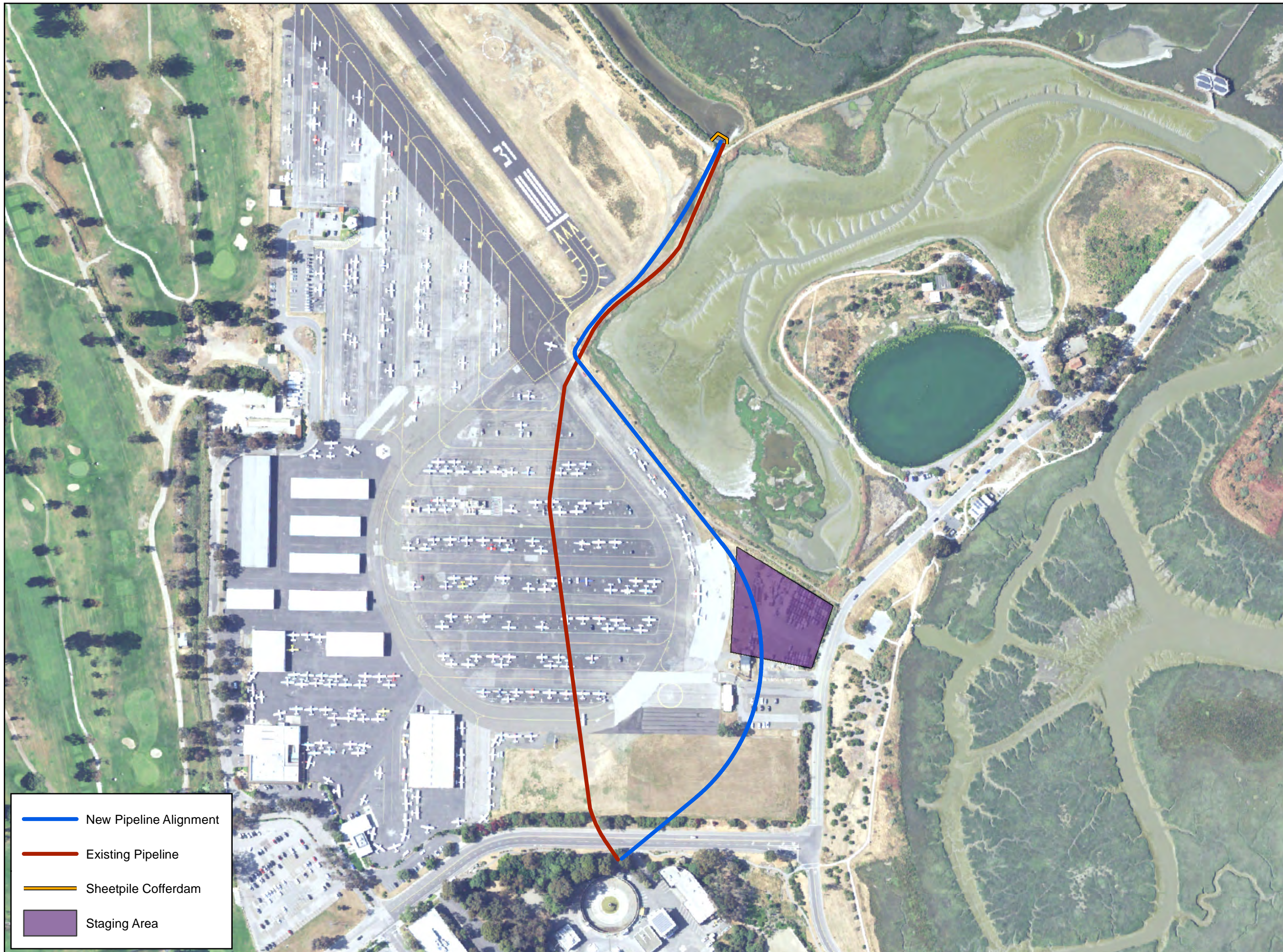
Figure 3. Proposed Pipeline Alignment
