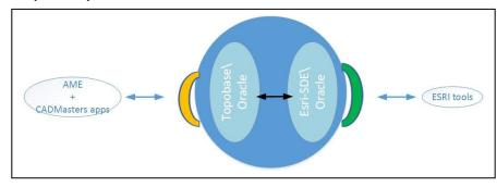
Once an ArcGIS platform is fully implemented as shown in the proposed system architecture diagram, data will be synchronized between CAD and Esri data stores using FME ETLs.
