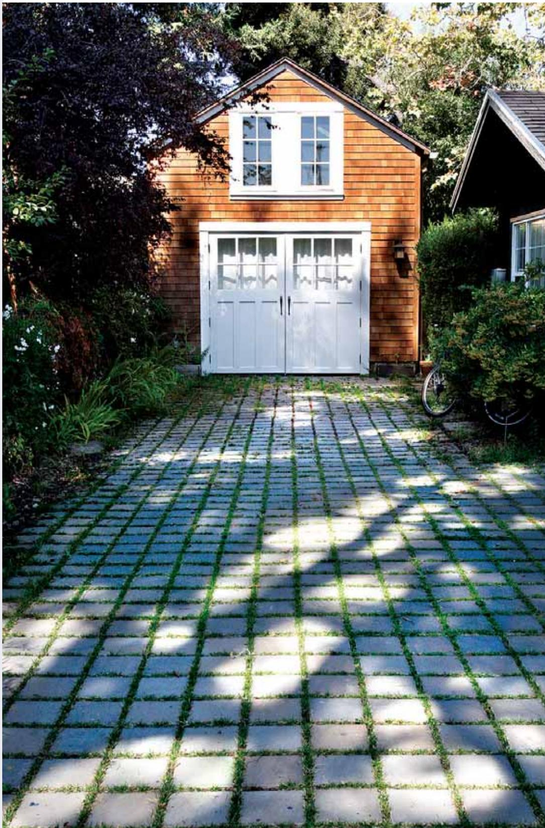
Cutting down on impervious area, by eliminating large expanses of paved driveway, is one way to reduce storm-water runoff. Hiromi and Kurt Kietly replaced their Homer Avenue asphalt driveway with permeable pavers.
