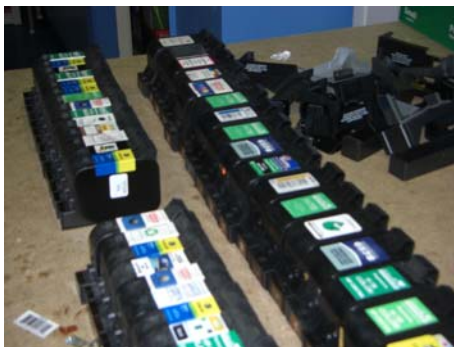
Ink cartridges are cleaned and refilled with water-based inks on premises
